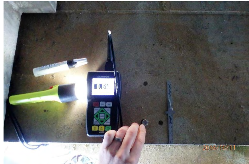
Bent 3 piling cap ultrasonic thickness testing (515 mils min)
